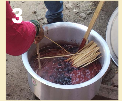
Dyeing & soaking – bamboo strips are soaked in heated dye solution to absorb color, then washed to remove excess.
