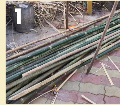
Selecting Bamboo – Mature bamboo is carefully chosen and split into fine strips.
