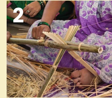
Preparing the Strips – The strips are cleaned and smoothed to make them flexible.
